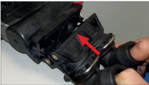
Position the previously disassembled connection block on the block with the bypass valve.
