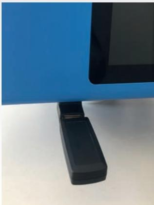
Put the Wifi USB stick with the angle adapter into the USP port of the controller.
