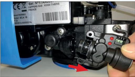
Remove the chlorinator cell.
