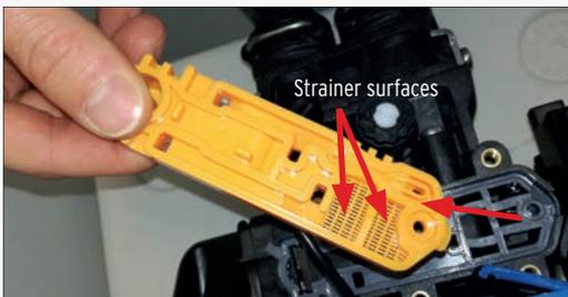
Remove the holder and clean especially the strainer surfaces with cold clear water.
