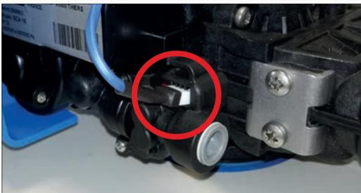
Plug the connecting cable in the chlorinator cell.
