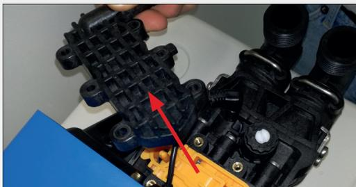
Remove the holder of the sealing kit.
