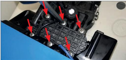
Remove the six screws with a screwdriver.
